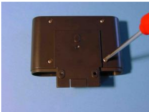
Figure: Opening the OPUS10 to change the battery
